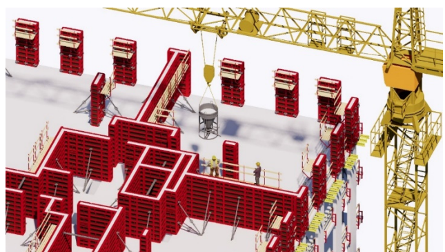
Fig. 3 – Modeling of the technological process (concreting)
